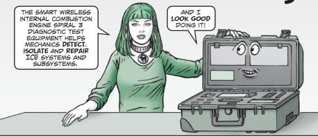
The SWICE SP 3 connects with the Maintenance Support Device version 3 (MSD-V3) and the equipment tested to perform standard voltage, current, resistance, pressure and rpms and capture digital diagnostic data.
