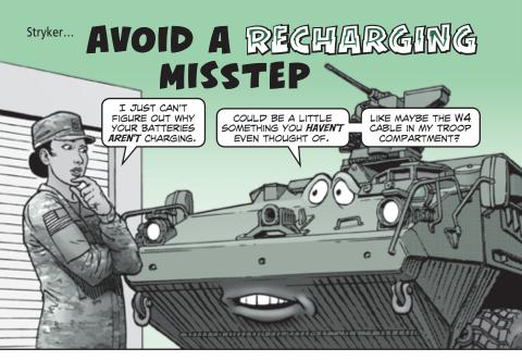
Mechanics, figuring out why a Stryker's batteries aren't charging can be tricky and time consuming. But you might save yourself some trouble by making the W4 cable inside the troop compartment one of your first checks.
